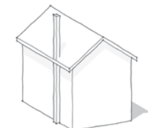
Not Proportional Chimney - notice the size is too narrow and thin. This is out of proportion.
