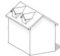
New Dormers must be either consistent or complementary to the existing roof form, such as these gable dormers.
