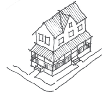
Changes can be made to address side walls in the event they are not attractive or do not address the street or open space well. These can include adding wings, dormers or porches.
