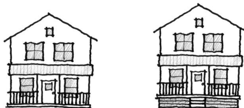
There should be no slab-on-grade foundations. The foundation height should be consistent with the foundations of adjacent houses. In general, first floors shall be set so that 16 to 24” of foundation is exposed.
